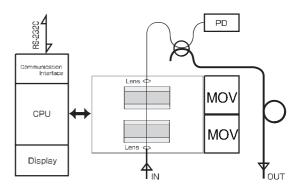
The OVA-60 incorporates two highly linear neutral density filters. These are mounted on independently controlled sliders and allows for customization of both the attenuation range and resolution. In the standard configuration an element with 40dB maximum attenuation is mounted on one slider, and an element with 20dB maximum attenuation is mounted on the second. This combination achieves a high 60dB attenuation range whilst maintaining resolution of better than 0.01dB.
